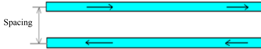
Figure 4.1: Two-Wire Transmission Line
